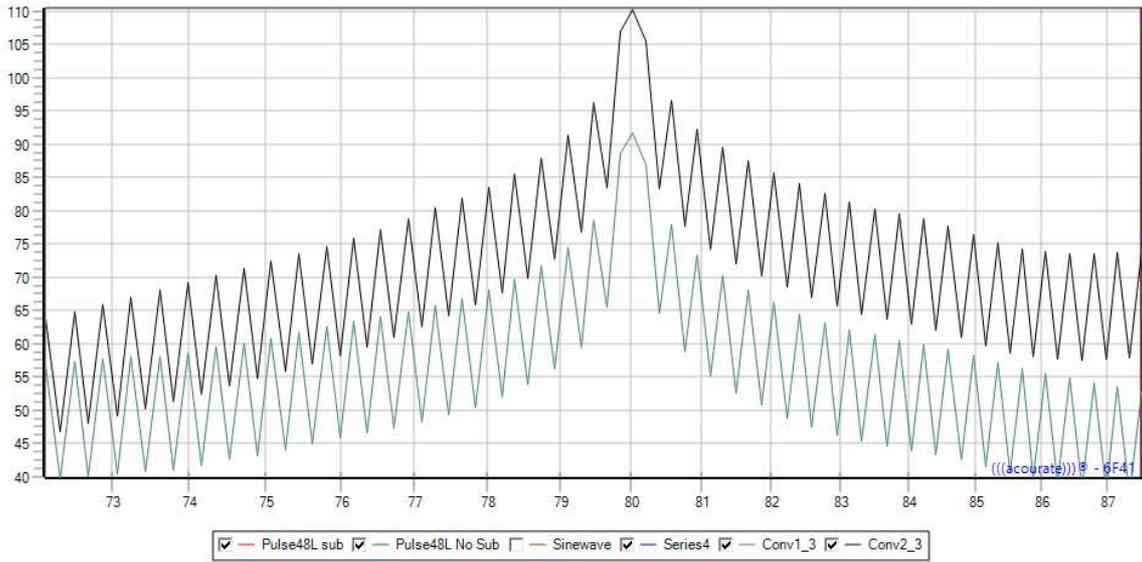
A zoom of the frequency shows that the sub signal is about -18 dB lower. So we apply a gain of 18 dB and get
