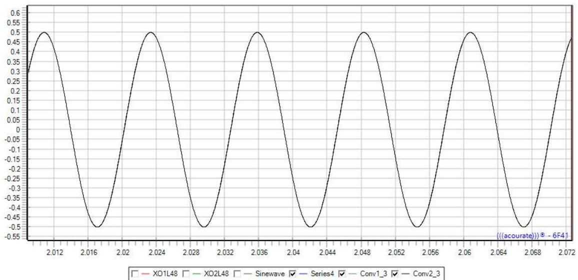
Indeed in the perfect world both convolution results match in phase (because of the linear phase filters) and amplitude (0.5 = -6 dB point @ 80 Hz). So in the steady state we expect the results to be in phase, otherwise we do not match the timing requirements.
