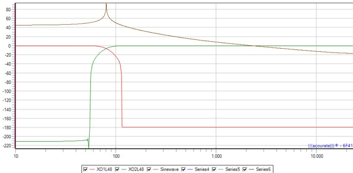
The picture shows the frequency response of a lowpass and a highpass crossover NT2 with a corner frequency is 80 Hz. Furthermore the picture shows an 80 Hz sinewave created by Generate – Sinewave – 80 Hz
