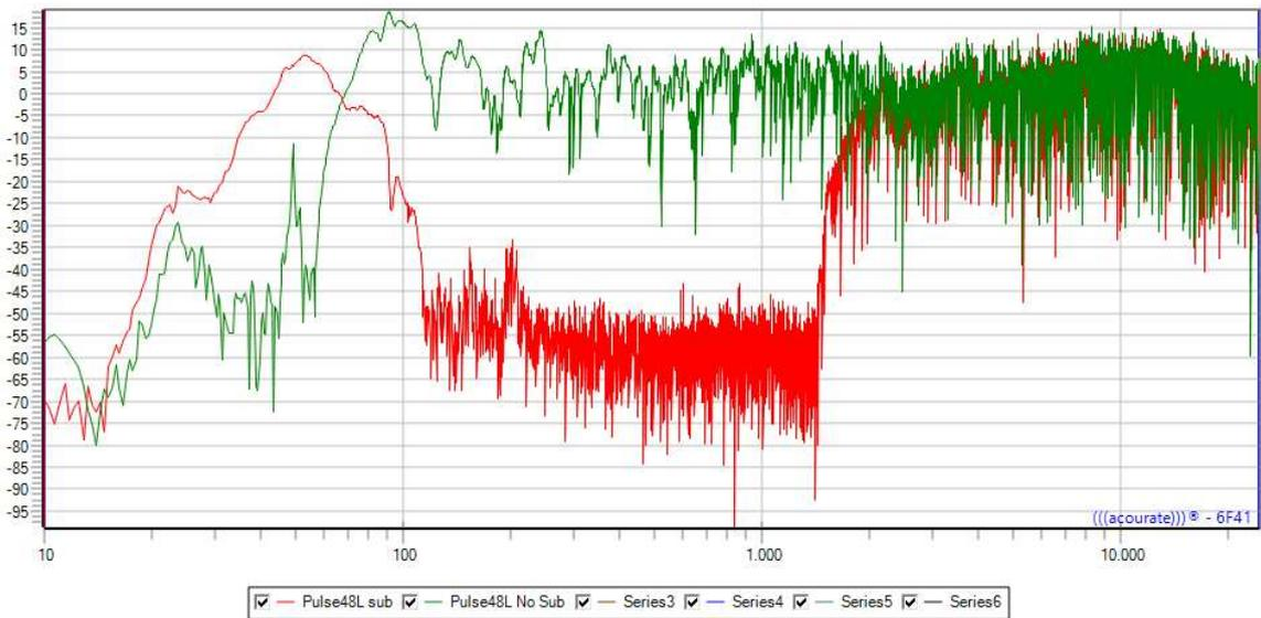
The picture shows two frequency responses. The green one is the main speaker without subwoofer. The red one is the subwoofer plus the main speaker treated by a highpass. This allows the pulse responses to be perfectly time aligned by the high frequency content in the responses. Because the high frequency content creates a peak with a high amplitude. This is demonstrated by the next picture in time domain:
