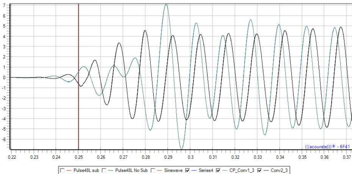
This definitely looks better for the expected transition zone. But now we also detect that the steady state behaviour is not optimal as the signals run out of phase. We also see some reflection influence at time  $\sim 0.27$ . So we must make a decision about a compromise. We can rotate the sub by 131 samples to the right and get
