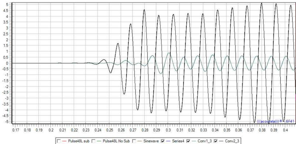
Well, we clearly recognize a pretty low signal amplitude of the subwoofer in comparison to the main speaker. A first approach would be to adjust the gain of the subwoofer in relation to the main speaker, if possible. We can even adjust this by applying some gain to the measurements.
