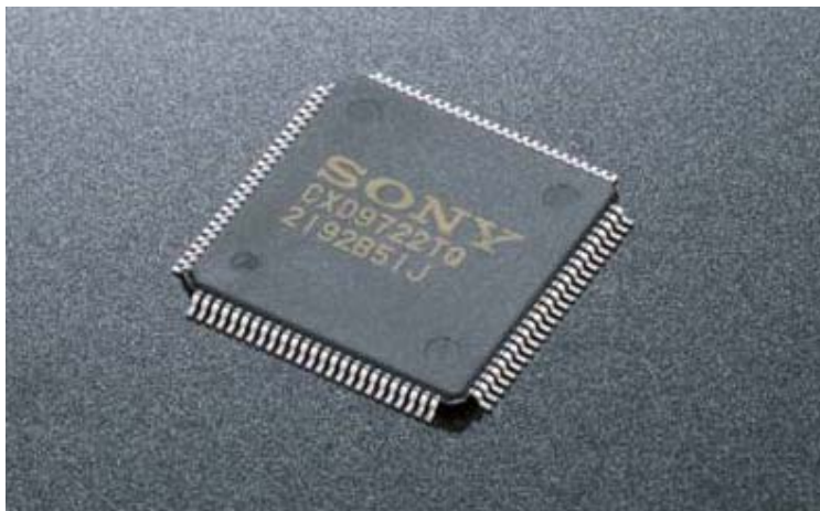
The STR-DA5000ES performs Lip Sync with another Sony Large Scale Integrated circuit, the CXD9722.
