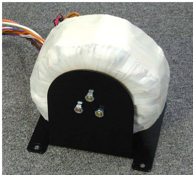
The extraordinary size and weight of the STR-DA9000ES receiver is explained in part by the size and weight of this toroidal-core power transformer.
