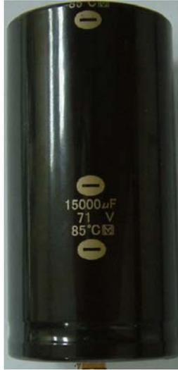
*Sometimes size does matter, as in the oversized filter capacitors of Sony's STR-DA3100ES.*
