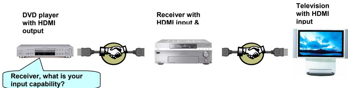
The receiver must then communicate with the television and mediate the content exchange for the entire system. The receiver automatically passes through the television's video requirements back to the source component. In the case of this illustration, the television is asking for 720p.
