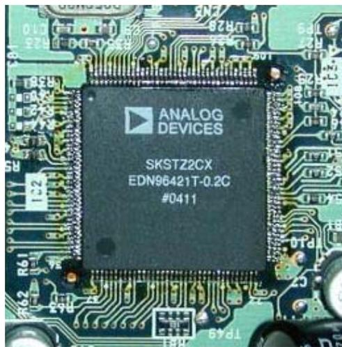
*The Analog Devices SHARC DSP achieves true 32-bit floating-point processing, for exceptional precision.*
