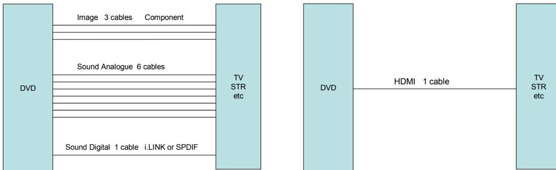
*Before HDMI (left), you needed nine cables to get component video and 5.1-channel analog audio from your DVD player and into your receiver. If you wanted digital audio as well, that would mean a tenth cable. HDMI conveys both video and audio with full resolution and digital precision—all on a single cable!*
