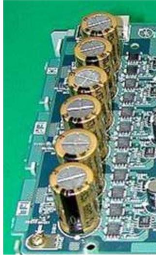
*A detail of the power amplifier circuit board of the STR-DA7100ES. The twelve black chips are the MOS FET output transistors for three channels (4 MOS FETs per channel).*
