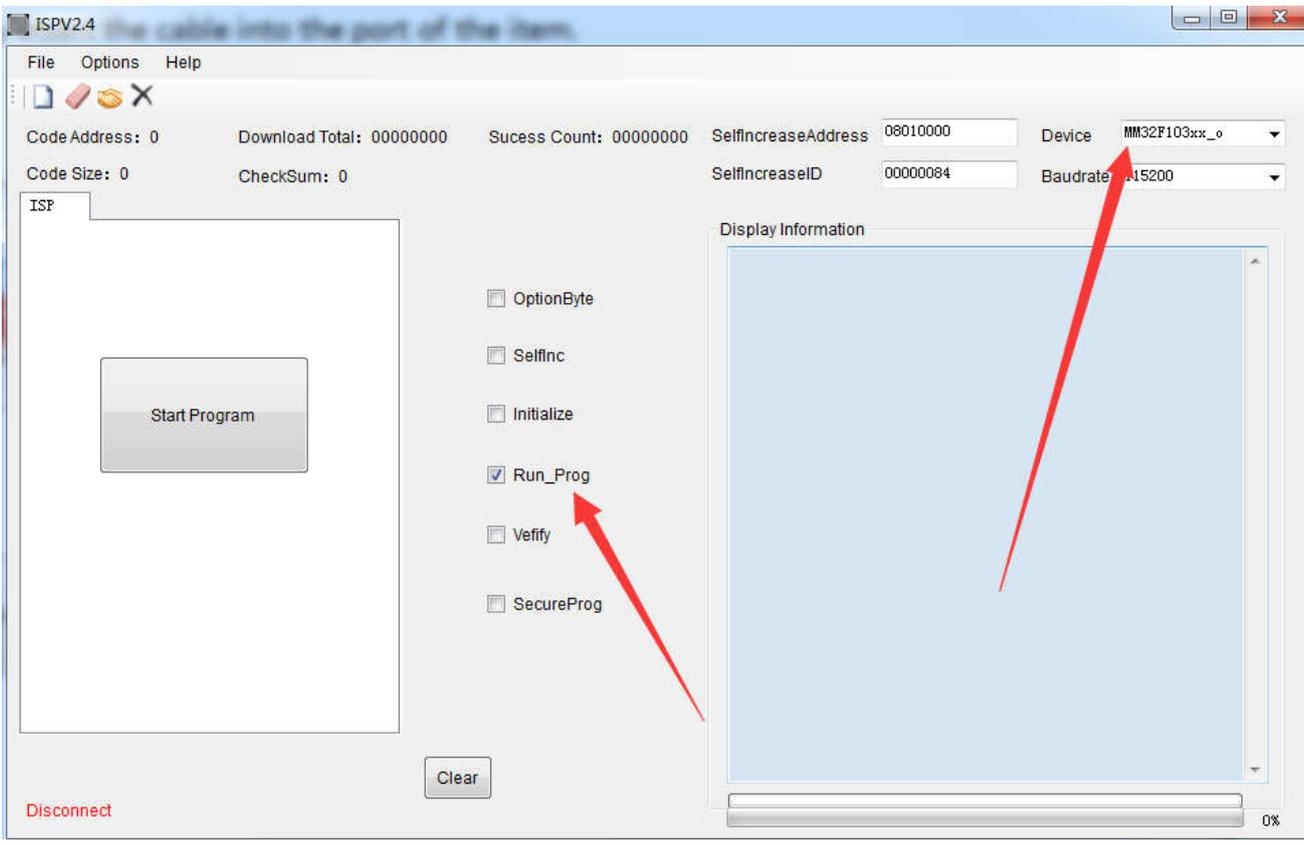
5 ) Operation according to picture show. File → Open →Select the firmware you want to update “SMSL\_D300\_XXX.hex” , then wait for the program to load the firmware, this process takes about 30 seconds.
