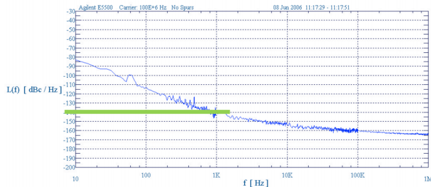
Figure 7. SSB phase noise plot of a true ultra-low phase noise oscillator (model: Crystek CCHD-950).
