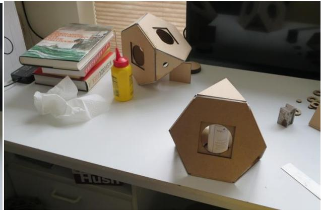
The material used is 4 mm MDF. The hexagons and triangles must be precise to size. In the absence of a saw table, I ordered the material from a laser cutting company. The baffles are held in place with adhesive tape and then folded together. The resulting v-seams are filled with wood glue. Also on the inside, all seams must be glued to get sufficient strength.
