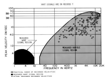
"the situation is actually worse than the considerations above imply when we come to play the record, because a further limitation exists on reproduced velocity when the stylus radius dimension exceeds the radius of the recorded curve" a stylus with an effective radius of 5µm (as do the best hyper-ellipticals etc.), will keep ahead of the limitations due to cutting at all recorded radii."
