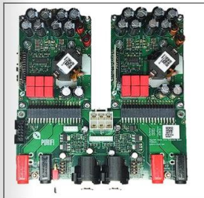
Photo 3: Purifi's EVAL1 system combines two 1ET400A power amplifier modules with a front end and control system, suitable for use as a stereo power amplifier.
