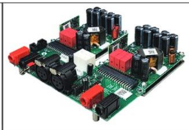
Photo 3: Purifi's EVAL1 system combines two 1ET400A power amplifier modules with a front end and control system, suitable for use as a stereo power amplifier.
